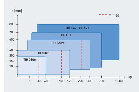
The comprehensive range of SKF induction heaters is suitable for most bearing heating applications. The chart gives general information on choosing an induction heater for bearing heating applications <sup>1)</sup>.
